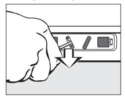
■ Insert a screwdriver into the notch of the left opening and pull downwards. The door will now open.
